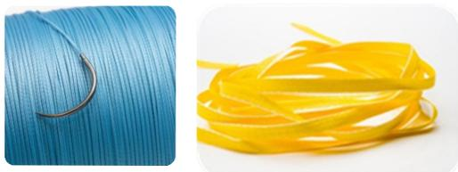
Figure 1: A braided suture made of Dyneema Purity® VG fiber containing Chromium-Cobalt-Aluminum Oxide (left) and a woven wire made of Dyneema Purity® RP fiber containing Bi<sub>2</sub>O<sub>3</sub> (right).
