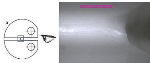
Figure 4. Left: schema showing viewing orientation to observe the notch root. Right: Video image of an XLK specimen tested at 1400 N showing void coalescence along the plane of fracture initiation.
