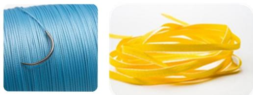
Figure 1: A braided suture made of Dyneema Purity® VG fiber containing Chromium-Cobalt-Aluminum Oxide (left) and a woven wire made of Dyneema Purity® RP fiber containing Bi<sub>2</sub>O<sub>3</sub> (right).
