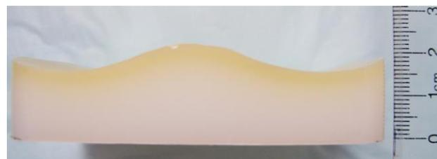
**Figure 2.** Side view of the consolidated contoured sample, condyle height 14 mm and eminence height 19 mm.
