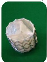
Figure 1 Stented heart valve made of fabric of UHMWPE fibers.
